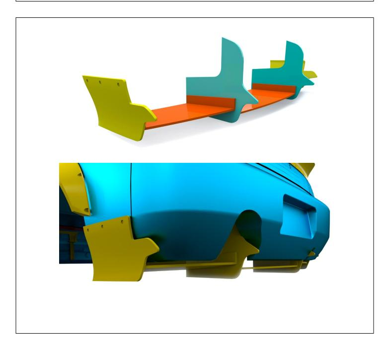
Attach the diffuser on both side of the body with screws.
