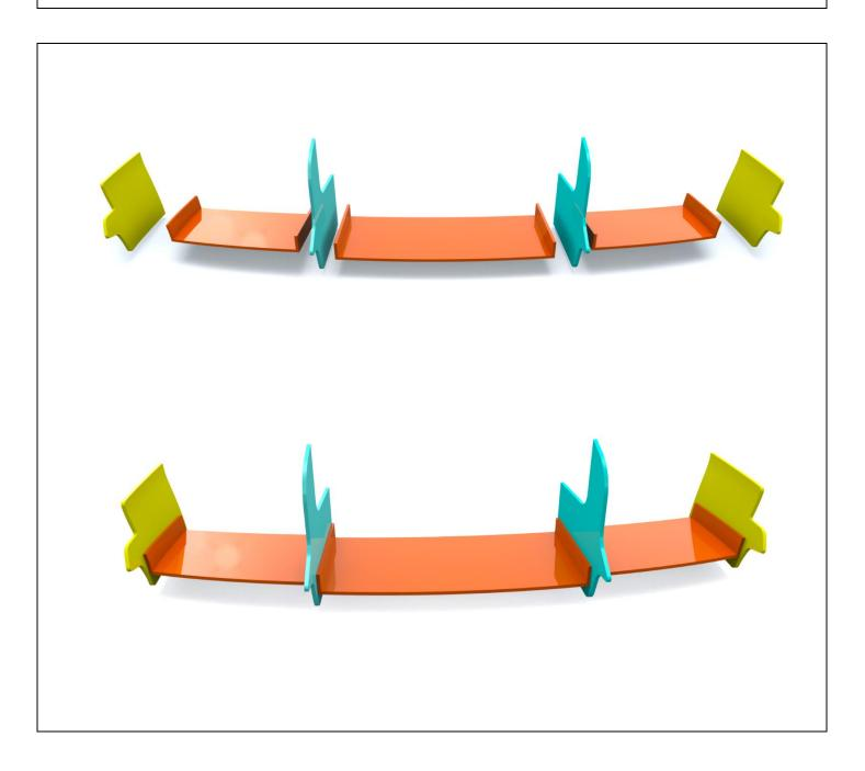
Glue the parts of the diffuser together.
